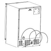
Locate the U-Line supplied garden hose fitting. Ensure the end of the copper tubing has been cut straight and free of burrs. Slide the compression nut and ferrule onto the copper tubing as shown. Push the assembly completely into the garden hose fitting and tighten using the two wrenches.
